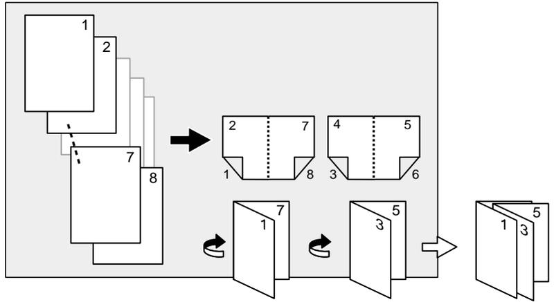
Magazine Mode allows you to make A4 or A5 size magazines from single- or double-sided originals.
